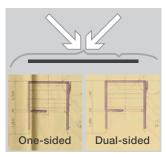
Contex CleanScan CIS The IQ Quattro Scanners are equipped with Contex CleanScan CIS modules which facilitate optical image quality with dual-sided LED lighting. This eliminates creases and folds in originals normally a challenge for CIS scanners, and thus provides clear, crisp scans every time.
